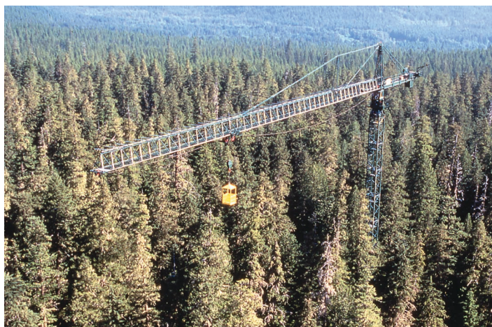
Figure 1. The forest canopy of the Pacific Northwest and the Wind River Canopy Crane Research Facility. The WRCCRF is one of several research sites specialized for studying the forest canopy. A construction crane lets researchers study the canopy from multiple viewpoints. Several researchers working with the Canopy Database Project use this crane site. (Photo courtesy of J. Franklin.)
