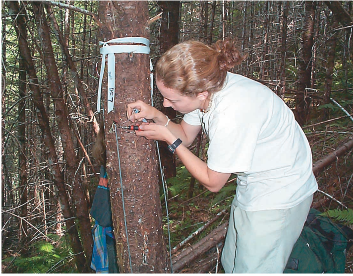
Figure 4. Part of a field installation for a study of environmental controls on ecosystem-scale physiological processes. A student is installing a sensor to continuously monitor the flow of water through the sapwood of a Douglas fir tree. (Photo courtesy of B. Bond.)
